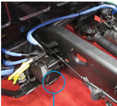
Sample location of medium duty application dosing system. Bosch Urea Filter located on underside of dosing system.
