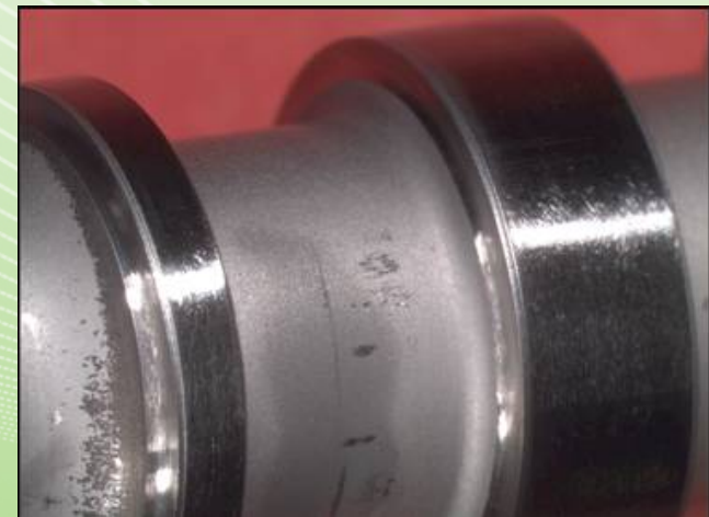
Worn edges of CVB Spool
